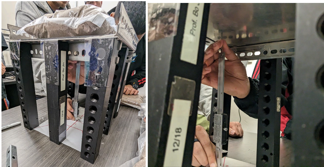
Figure 5:(A) AI plate deflection being measured (B): Vernier caliper used to measure deflection
